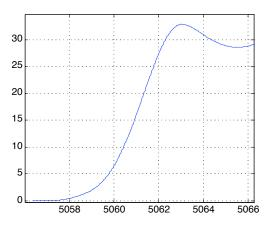
Fig. 10 Recorded altitude during an automatic takeoff and climb to a hover at 30 ft of altitude.
