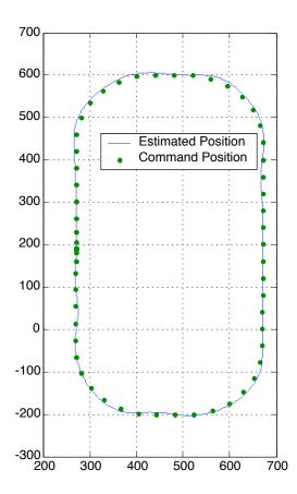
Fig. 8 Racetrack pattern flown at 40 ft/s starting and finishing in hover, commanded position plotted once per second
