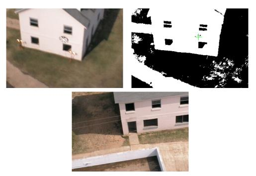
Fig. 14 (top) Typical image of symbol (black circle with white "X") used to automatically identify building, raw on left, a processed image with green "+" on symbol on right; (bottom) automatically selected opening to this building is the door in the center of the image.
