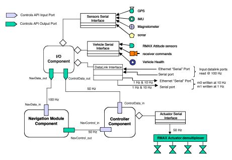
Fig. 7 Open Control Platform (OCP) implementation of baseline GTMax guidance, navigation, flight control, and communication.
