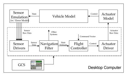
Fig. 5 Nominal software in the loop configuration.
