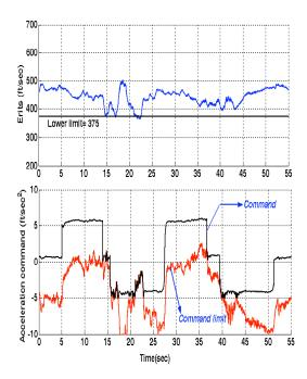
Fig. 12 Erits factor limit (a prediction of blade stall) is avoided by modifying the commanded trajectory acceleration.
