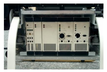
Fig. 2 Vibration isolated avionics module rack, from left to right: data link module, GPS module, computer module #1 (flight computer), and computer module #2 (auxiliary).
